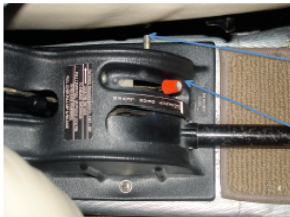
Auto Extension Lockout Pin
